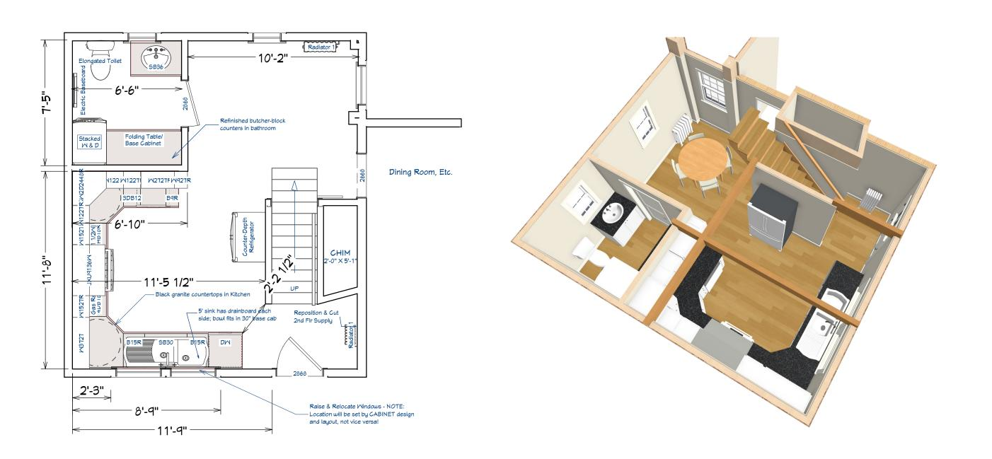
Floor Plan View, Dimensioned - Note that cabinet design & layout is DRAFT ONLY for illustrative purposes - need supplier design & costing
